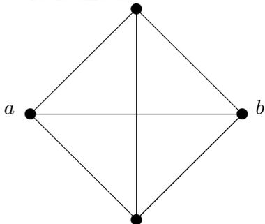
[5] What will happen with the effective resistance between  $a$  and  $b$ , if the direct link between  $a$  and  $b$  is removed? Formulate the general principle.
